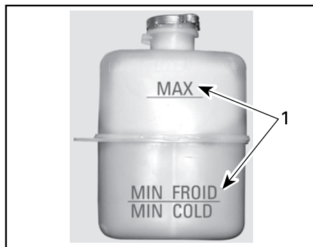
1. Level between marks when engine is cold
